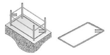
Figure 1: Steel reinforcement in columns – closed ties at close spacing improve the performance of columns under staring shaking of ground
