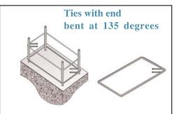
Figure 1: Steel reinforcement in colums- closed ties at close spacing-improve the performance of columns under strong shaking of ground.
